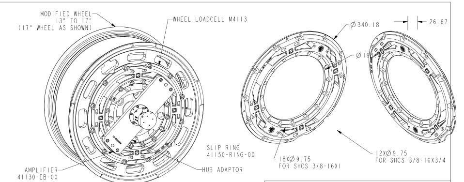
M4II3 Wheel Loadcell measures all wheel forces and moments. The six components of the total wheel load are structurally decoupled to provide independent outputs, so that post-data correction becomes unnecessary.
