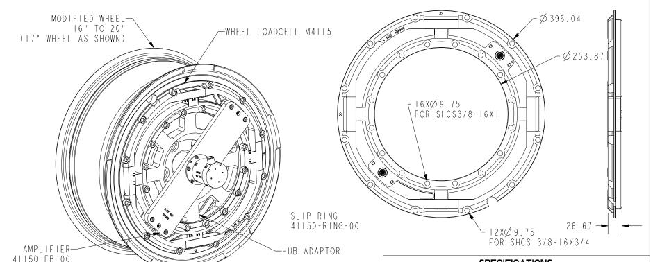
M4II5 Wheel Loadcell measures all wheel forces and moments. The six components of the total wheel load are structurally decoupled to provide independent outputs, so that post-data correction becomes unnecessary.
